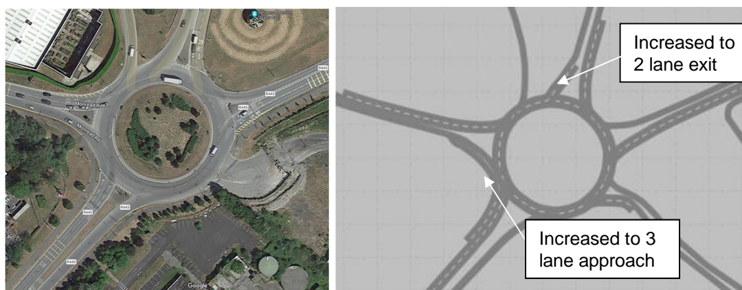
Figure 6-3: Fishery Lane Roundabout Existing Layout and Proposed Modifications
