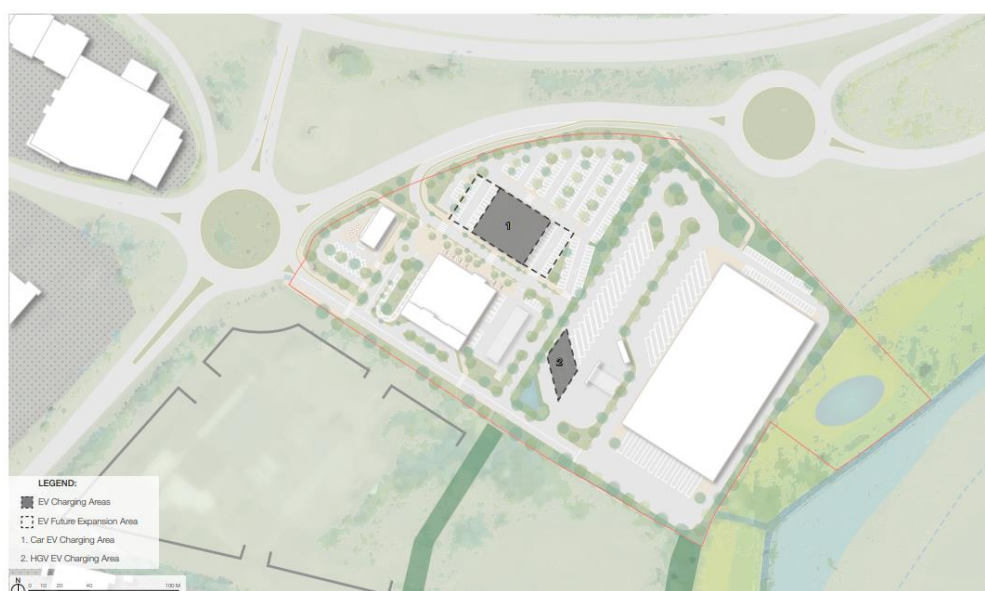
Figure 16. Car and HGV charging infrastructure in proposed development
