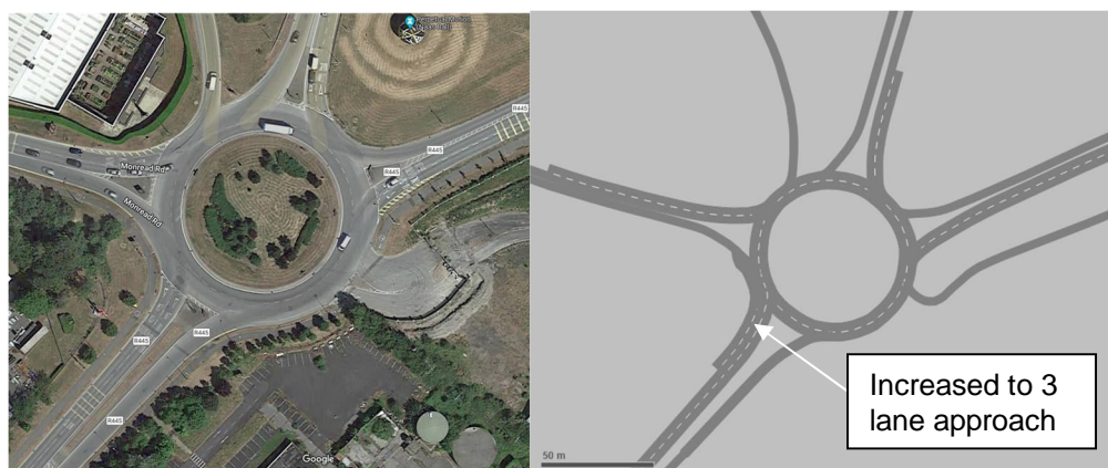
Figure 3-6: Maudlins Roundabout Existing Layout and Proposed Modifications
